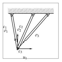
• *Remark:* For simplicity, strains are replaced by changes in length and stresses are tensions in the bars.
