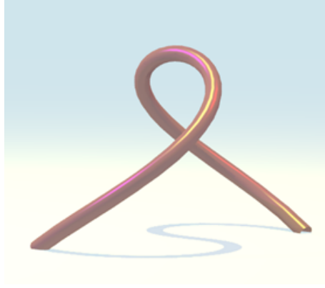
Figure 6: a loop of magnetic flux. With this shape, the magnetic helicity integral would equal -0.2\Phi^2 , where \Phi is the net magnetic flux along the loop, plus a contribution from internal twist of the field lines within the loop.
